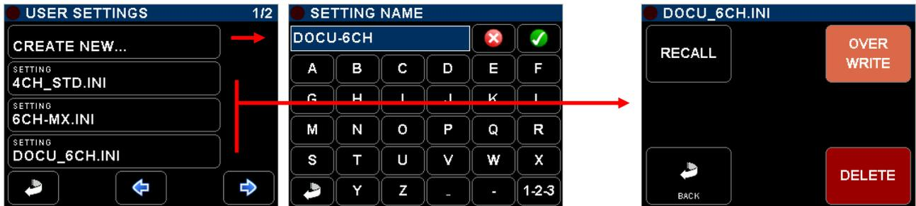
[CREATE NEW] Create a new User Setting file based on the actual configuration of the SX62R; a keyboard is posted to type a user settings name (max 8 characters); confirm with the green "check" key to save the setting.
