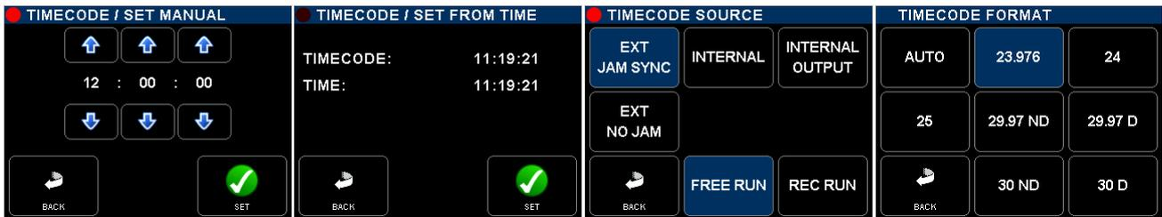
[SET MANUAL] set Hours : Minutes : Seconds manually, scroll the values with the Up & Down keys and then confirm with SET
