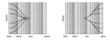
• **MF**: is a semi-parametric (sweep frequency) equalizer with a broad fixed bandwidth. ( Q Factor: -- ) The upper knob progressively adjusts the central frequency from 200 Hz to 8 kHz, the lower knob adjusts the gain of the filter.
